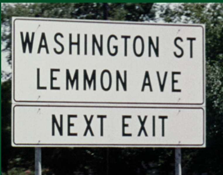
#17: This view shows a guide sign along Central Expressway with a white background and black lettering. The sign was probably a relic from the early days of Central Expressway. In January 1958 green was designated as the standard background color for signs on the Interstate Highway System and became the standard for all highways. Signs conforming to obsolete standards, such as this one, were replaced with signs having a green background.
