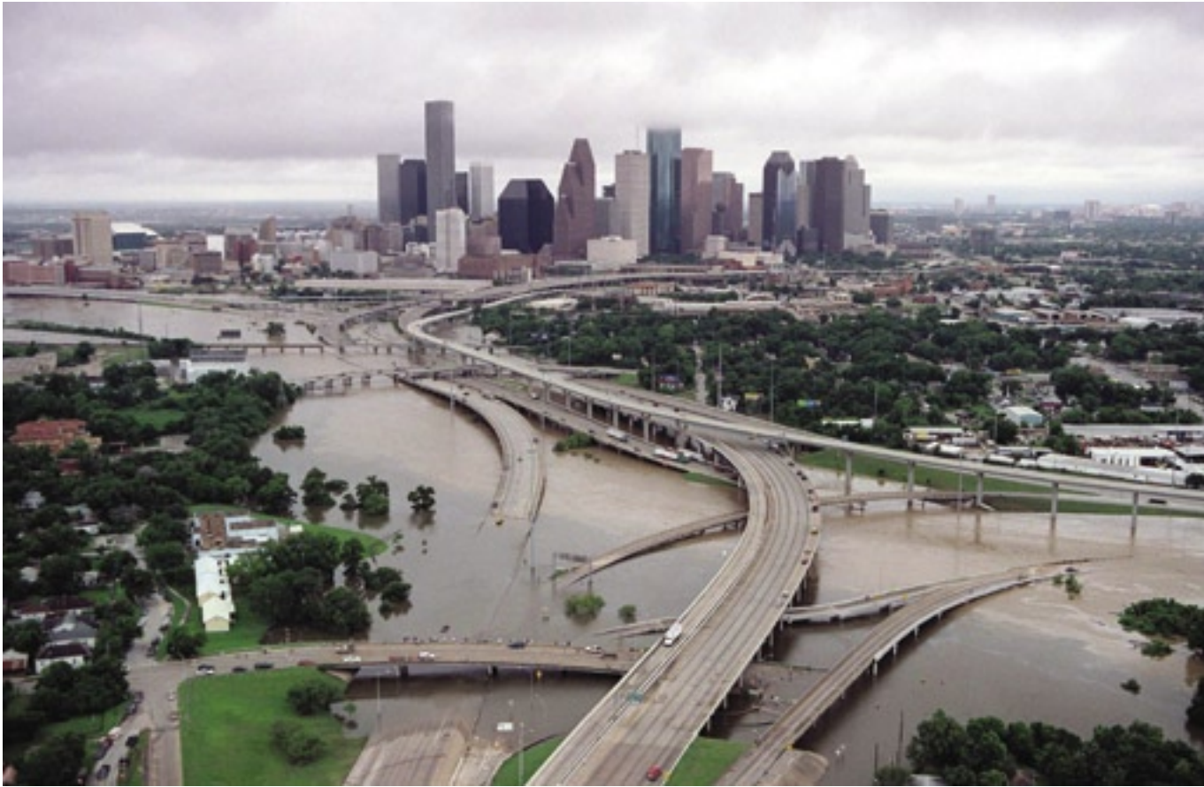
Houston's freeways turn into lakes: Tropical Storm Allison in June 2001 unleashed a major flood event, and Houston's freeways sustained some of the most dramatic flooding. Virtually all depressed freeways around Houston filled with water. Flooding along White Oak Bayou submerged much of the at-grade interchange of IH 45 and IH 10 north of downtown, shown above in a photo taken June 9, 2001. (Photo: Houston Chronicle )
